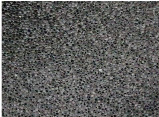
Figure 3.3.: Close up of the analyzed graphite foam
