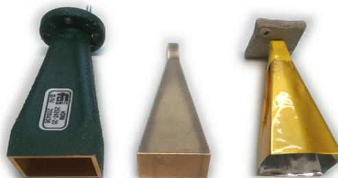
Figure 4.2.: Brass gain horn (left), negative (center), Kapton gain horn (right)
